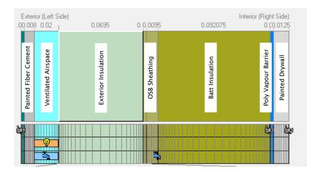
To simulate the drying potential, the initial moisture content of the OSB sheathing was saturated for a thin 3 mm layer near the exterior surface while the remainder of the sheathing was in equilibrium with 80% RH.
